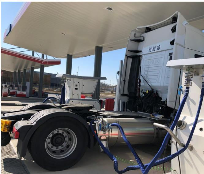
This picture shows the connection from the LNG dispenser to the LNG tank of the vehicle. Procedure is different depending on the type of truck
